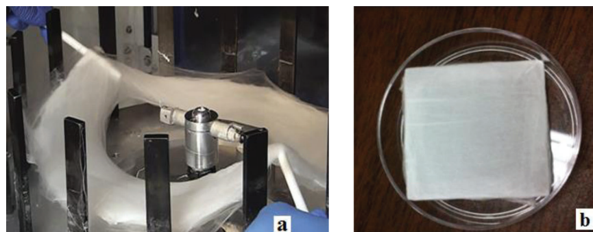
FIG. 1. (Color online) (a) Manufacture of Nylon 6 nanofibers using the forcespinning method (prototype system). (b) Pristine Nylon 6 nonwoven mat collected on square frames.
