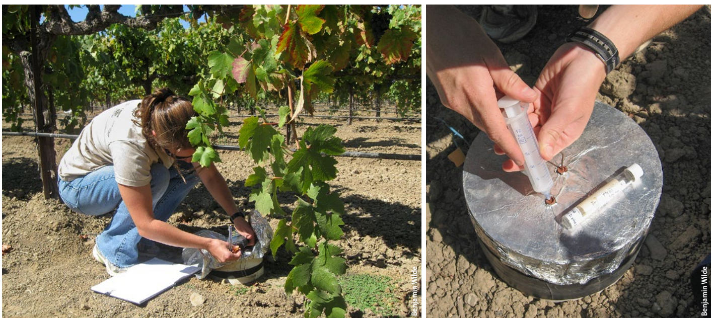
Author Gina Garland (left) records chamber temperatures and (right) takes chamber gas samples in a vineyard.
