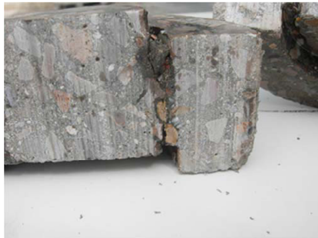
Figure 4: Fracture plane in confined test specimen, note the displaced aggregate which has been cut through in two pieces by a sensibly straight crack.
