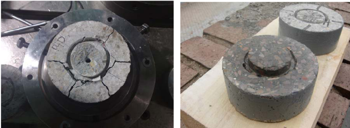
Figure 3: State of specimen after the unconfined test, with large fully developed radial cracks (left), and circumferential cracks with displaced core in a specimen tested under confining pressure of 8 MPa (right).
