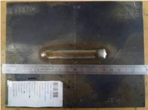
Figure 2: Picture of the top surface of the plate after welding
