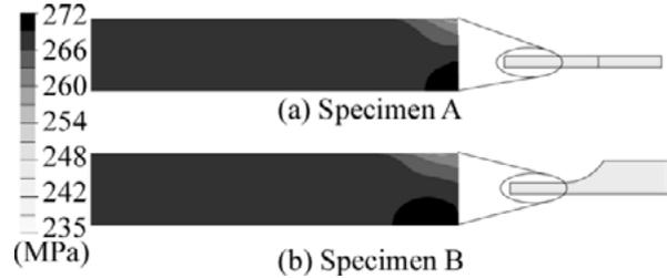
Figure 12: Axial stress distribution patterns in parallel part
