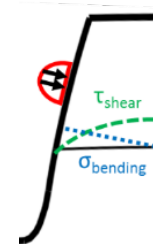
Figure 4: Tooth shear stresses and bending stresses
