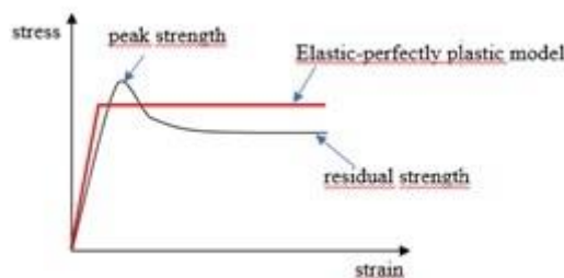
Figure 1: Characteristic stress-strain curve of soil
