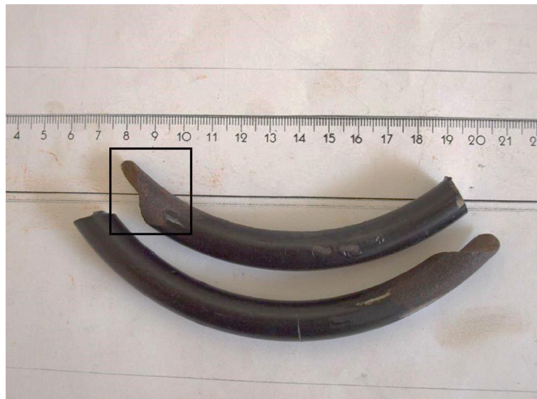
Figure 2: Specimens extracted from failed coil spring
