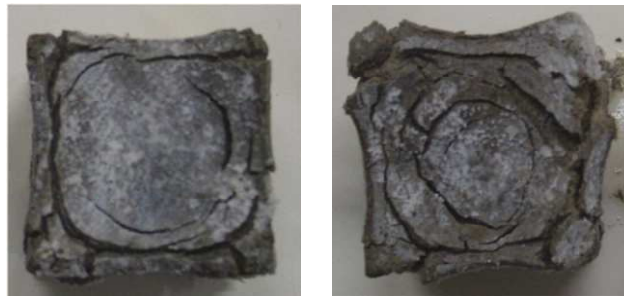
Figure 1: Cubic mortar specimen under the effects of the external magnesium sulfate attack at 360 days [2]
