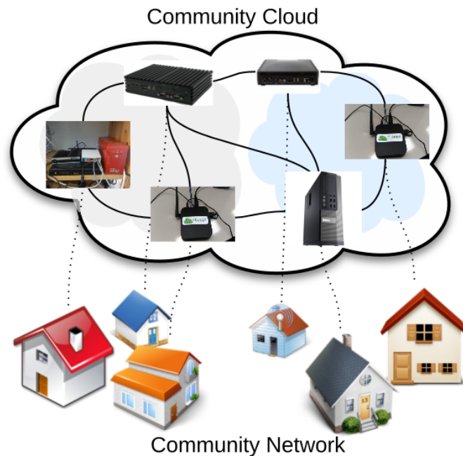
Figure 1: Edge community cloud in Guifi.net, running the Cloudy distribution on heterogeneous hardware.
