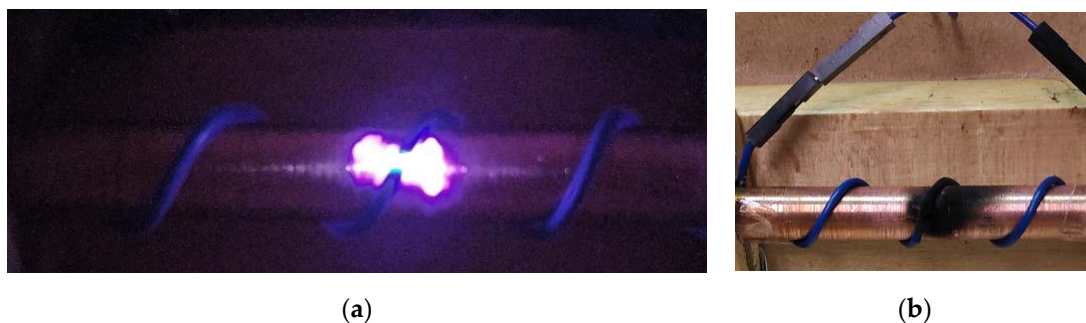
Figure 1. (a) Initial corona discharge at 10 kPa under 600 V–50 Hz. (b) Effect of arc tracking in a conductor.
