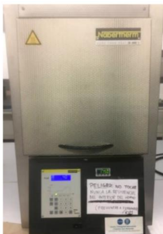
Figure 3.10. Nabatherm furnace used to sinter the samples.
