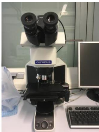
Figure 3.16. OM used during this Master's thesis.
