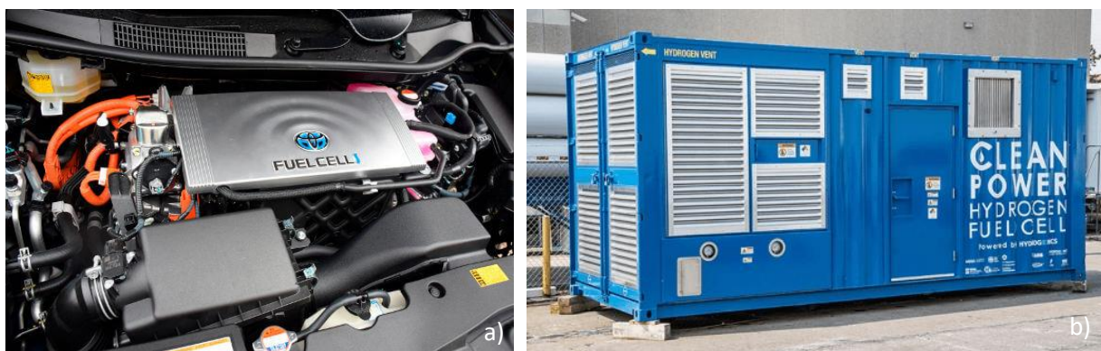
Figure 1.8. Different applications of fuel cells; a) Fuel cell in the Toyota Mirai model [6] and, b) a fuel cell for ships as part of a maritime project for the U.S. Department of Energy [7].
