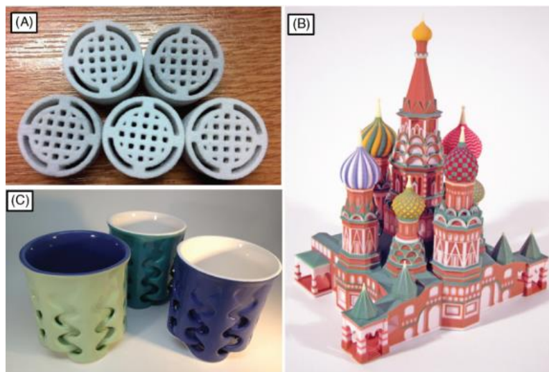
Figure 1.12. Examples of powder bed binder jet/inkjet 3D printed parts [16].
