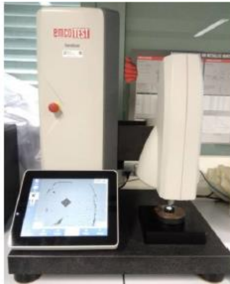
Figure 3.20. Vickers hardness machine EMCO-TEST Durascan.
