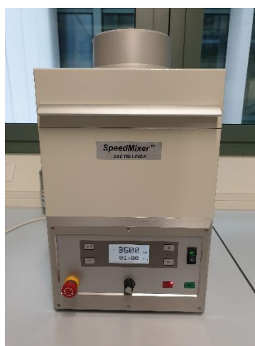
Figure 3.3. SpeedMixer used to mix the hydrogel and ceramic paste.
