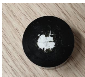
Figure 3.12. Destroyed embedded sample in Bakelite.
