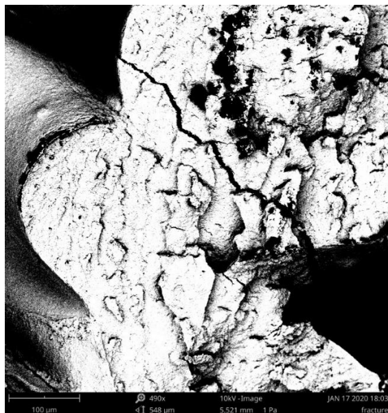
Figure 4.16. SEM image of a tubular 3D printed sample (scale of 100 \mu\text{m} ).
