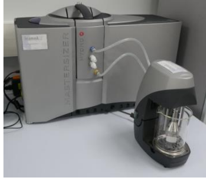
Figure 3.4. Mastersizer 3000 used during this Master's thesis.
