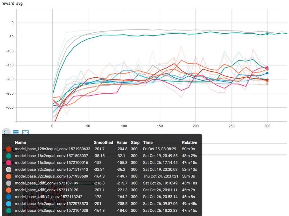
Figure 0.4. Average reward traces for all the tested models according to Table 0.2. on Map02. All the traces represented contain the models set with two identical convolutional layers with 16 neurons (on green – 16x2equal_conv), with 32 neurons (on grey - 32x2equal_conv), with 64 neurons (on light blue - 64x2equal_conv), the models set with three identical convolutional layers with 16 neurons (pink - 16x3equal_conv), 32 neurons (on orange – 32x3equal_conv), 64 neurons (green – 64x3equal_conv), 128 neurons (red – 128x3equal_conv), the model set with three convolutional layers each one with 16, 32 and 64 neurons respectively (on grey – 3diff_conv), the model set with four convolutional layers each one with 16, 32, 32 and 64 neurons respectively (on orange – 4diff_conv) and the model set with four convolutional layers each one with 32, 32, 64 and 64 neurons respectively (on dark blue – 4diff2_conv).
