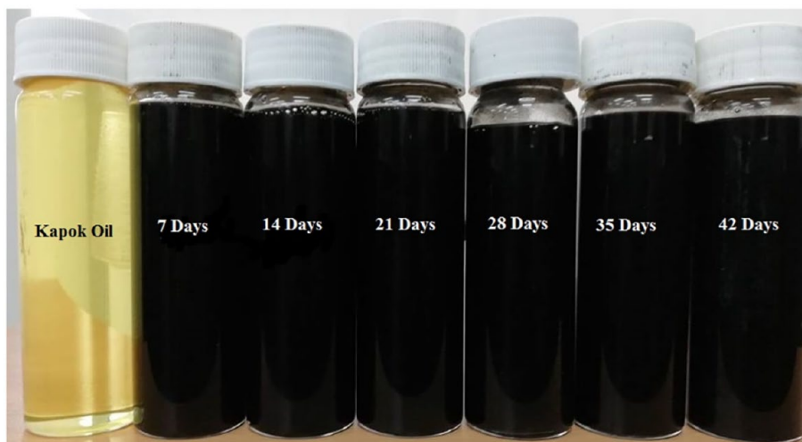
Fig. 5. Visual photographs of MWCNTs-Kapok seed oil based nanofluid samples after an interval of time.
