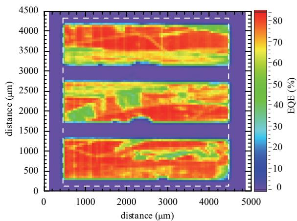
**Figure 3.** LBIC measurement and EQE mapping of the solar cell. Only the emitter regions are collecting carriers.
