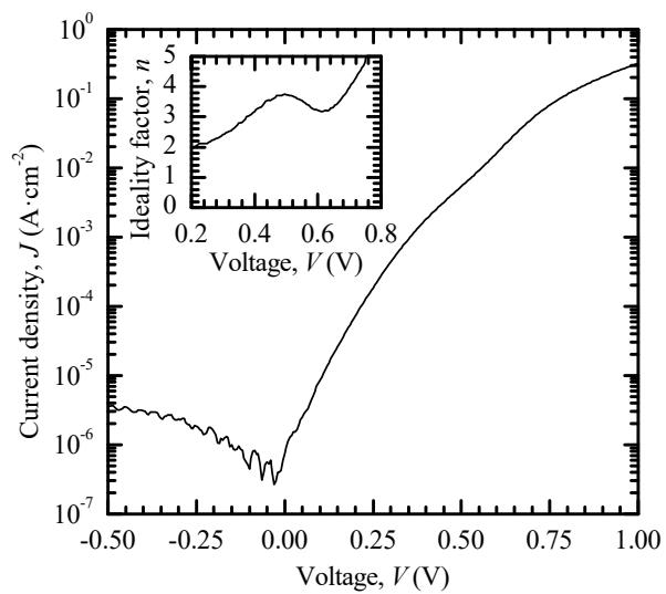
**Figure 2.** Dark J-V curve of the finished solar cell. (inset) Local ideality factor calculated applying equation (1).
