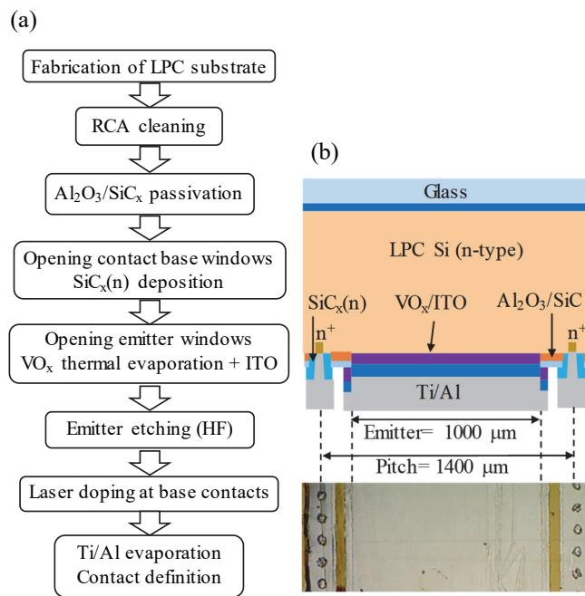
**Figure 1.**(a) Fabrication process of the solar cells; (b) sketch of the cross-section and microscopic image of the fingers at the final device.
