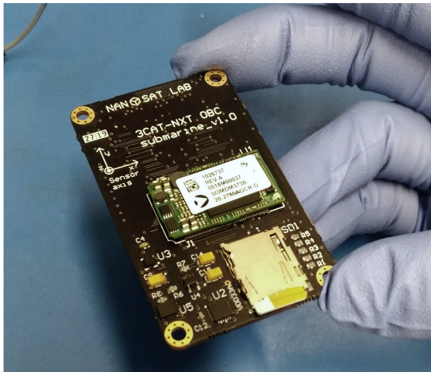
Figure 2.30: Submarine PCB finished with all the components soldered and the Torpedo SoM and µSD plugged
