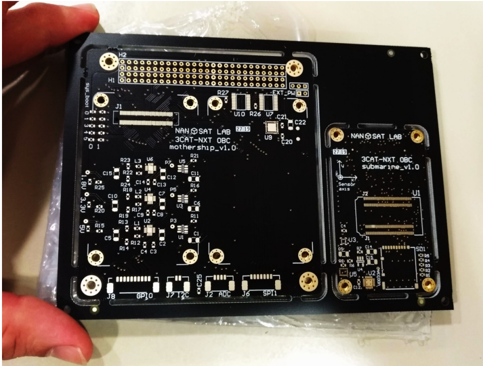
Figure 2.27: The two PCB boards just arrived from the manufacturer in a same panel
