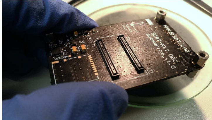
Figure 2.29: Both 100-pin connector soldered
