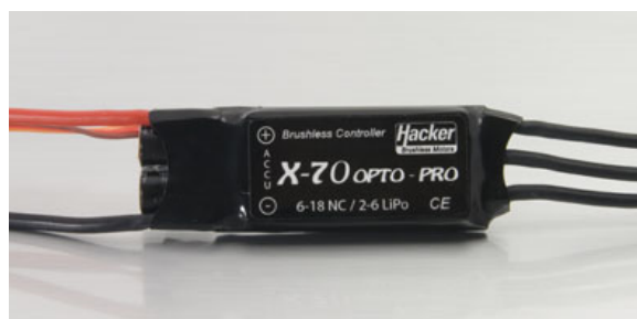
Figure 2.71: ESC X-70 OPTO-Pro [32]
