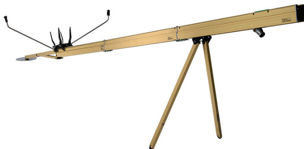
Figure 2.94: Assembled Pneumatic Catapult PL-40 [31]
