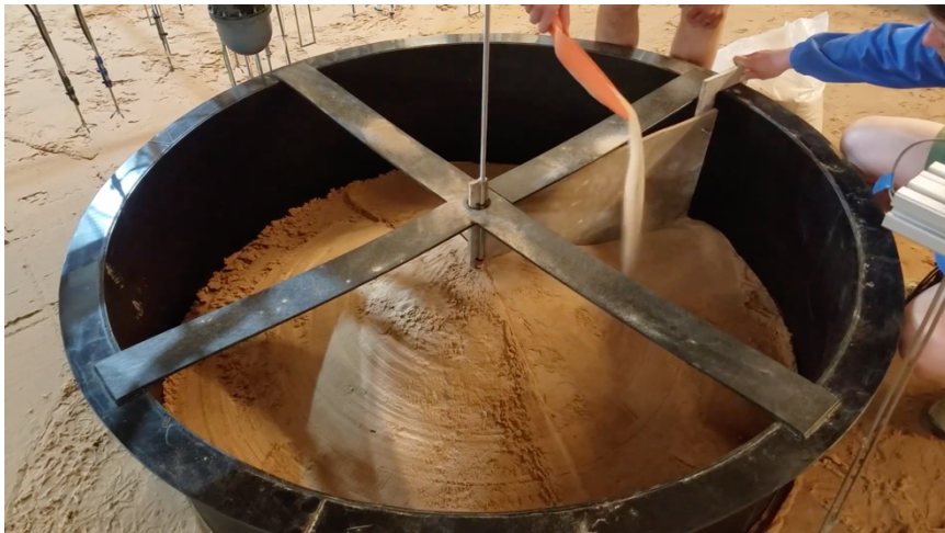
Fig. 2. Mound profile (top panel) and construction method in the flume.
