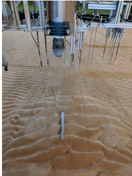
Fig. 8. Ripple patterns observed after Test 8 with waves and currents. Image facing the beach with a 30 cm ruler on the mound remains for scale.
