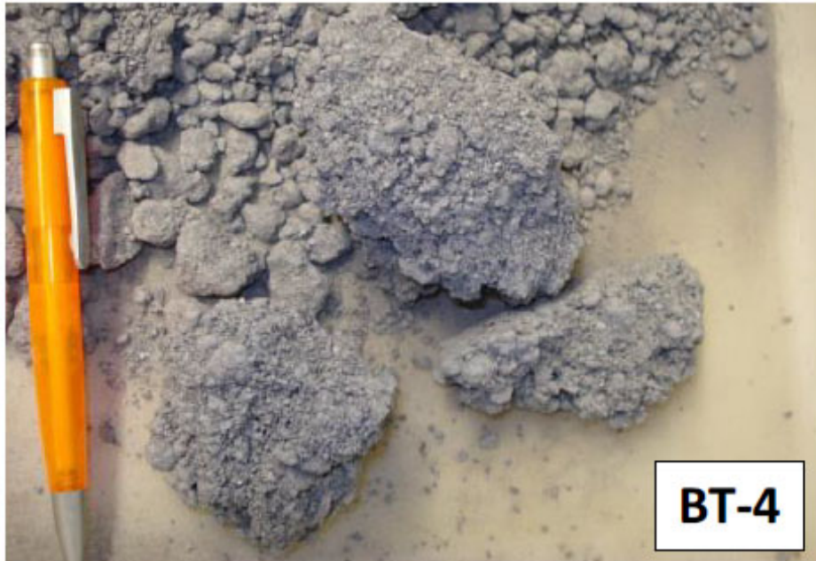
Fig. 6. Detail of the aggregate formation of the treated sample BT-4 and detail of isolated compacted agglomerates.
