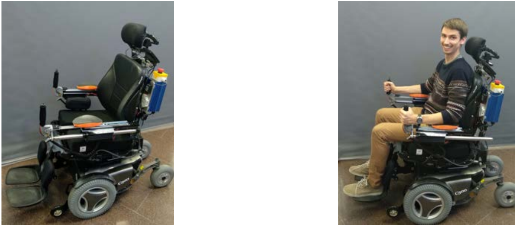
Figure 5. Picture of the Robotic MOVit, which consists of two robotic arm supports with linear actuators that replace the armrests of the wheelchair.
