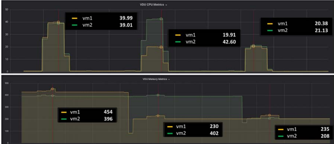
Figure 12. CPU (top) average usage [%] and RAM (bottom) consumption [MB] on VM1/VM2 as seen in Grafana dashboard.
