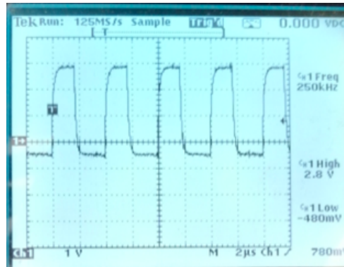
Figure 36: CH1: PWM signal sent by the CPU board to the inverter driver board. (1 V/div, 2 us/div).
