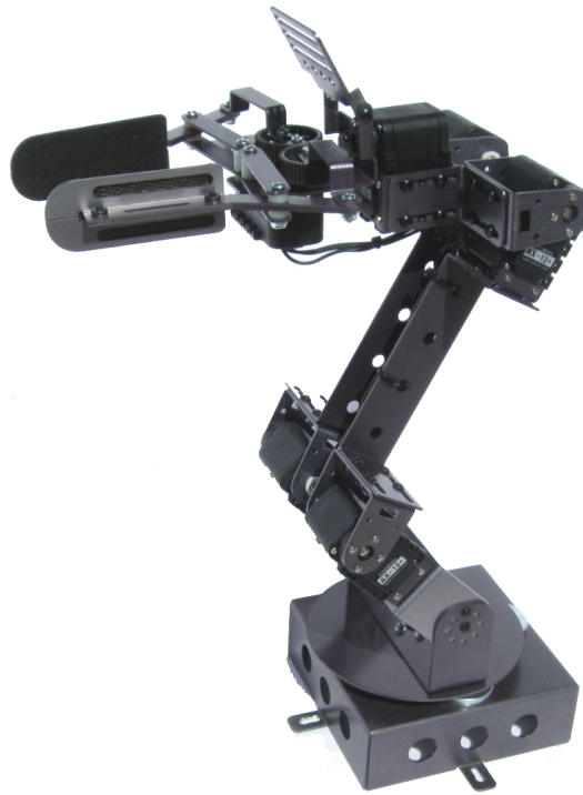
Figure 1.2: AX-18 Smart Industrial Robotic Arm used in this project.
