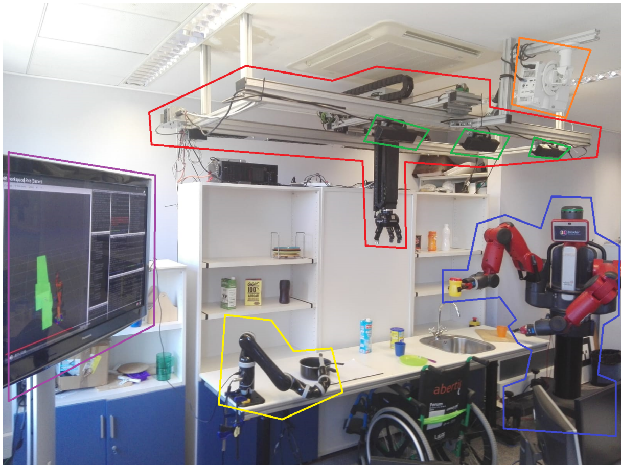
Figure 5.1: General view of the laboratory with the kitchen furniture and the robotic system.
