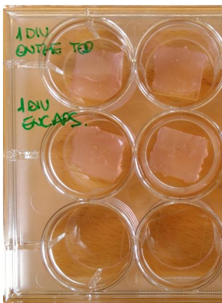
Figure 9: Glass surfaces where hydrogel and cells are adhered to make the process of application of teh live/dead assay and its analyses with the confocal microscope easier.
