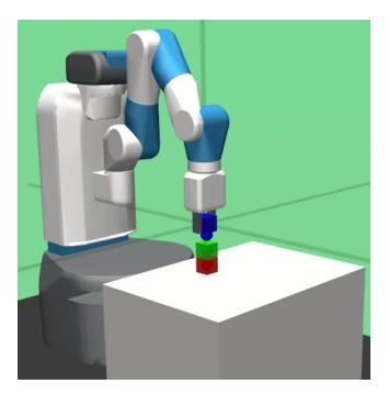
Figure 1.2: Fetch arm stack 3 blocks.
