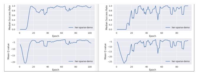
Figure 3.4: Network size comparison, left. 4 hidden layers, right. 3 hidden layers
