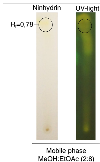
Figure 1. Thin layer chromatography (TLC) showing organic fraction with antimicrobial activity from Streptomyces sp. So13.3 crude extract against MRSA and S. aureus ATCC 25923. TLC was revealed by spraying with ninhydrin reagent or UV light exposition and TLC–bioautography assay on MRSA and S. aureus ATCC 25923 is shown. Active fraction of the crude extract in the TLC is shown with a circle selection (retardation factor ( R_f ) = 0.78).
