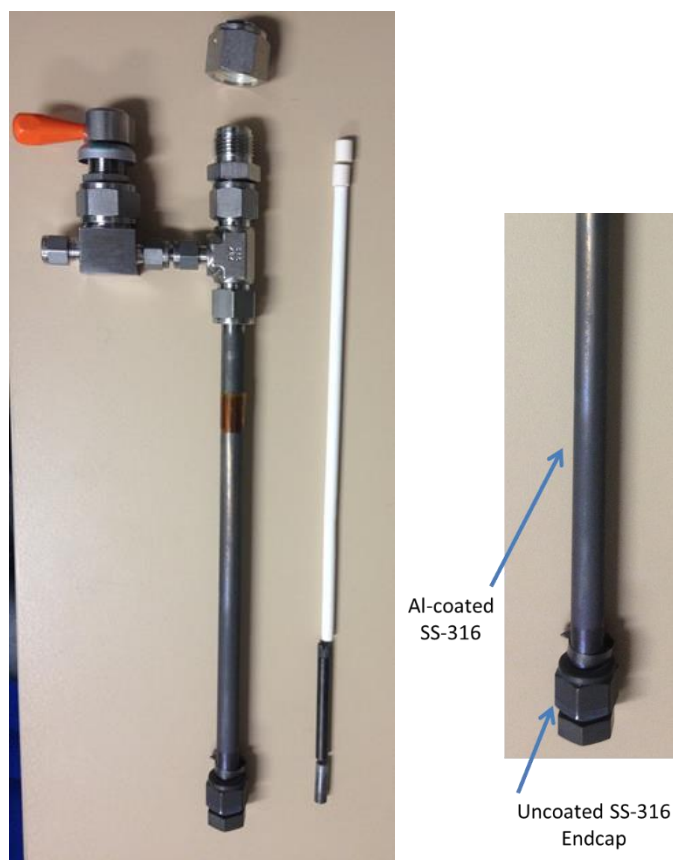
Figure 2-5: Picture of a SCR with aluminised tube used for sorption measurement at T \leq 700^{\circ}\text{C} .
