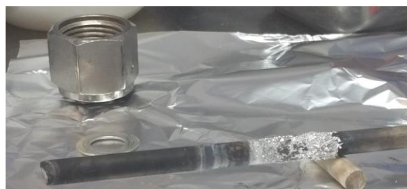
Figure 6-9: Photograph of Mg metal deposit on the alumina rod after TPD measurement.
