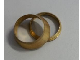
Figure 2-6: Pictures of the different ferrules tested to connect the \alpha -SiC tube to the Swagelok stainless steel connections.
