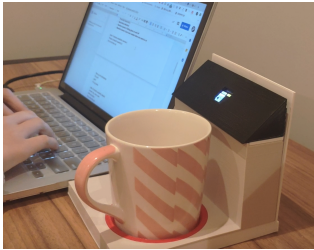
Figure 1: CoasterMe, a situated desktop widget that supports informal workplace awareness by detecting the presence of the user's cup. CoasterMe sends out a signal to a partner device to convey the user's presence at their desk, increasing awareness of availability and enhancing coordination.
