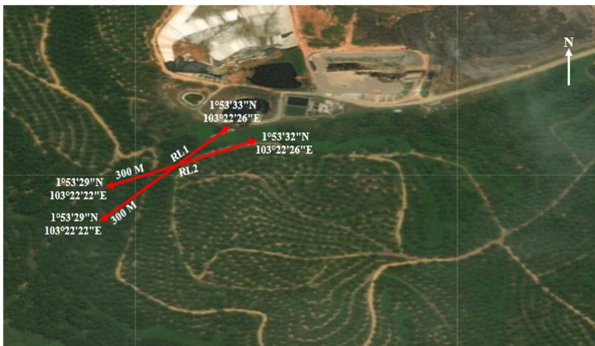
Figure 2. Entire location of resistivity lines (spread lines) conducted at Simpang Renggam Landfill, Johor.
