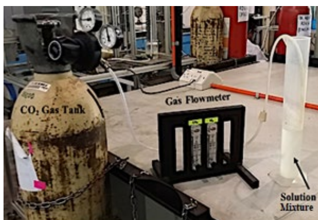
Fig 1. Experimental setup of the foam stability at static bulk scale with the gas flow controller for air flow control
