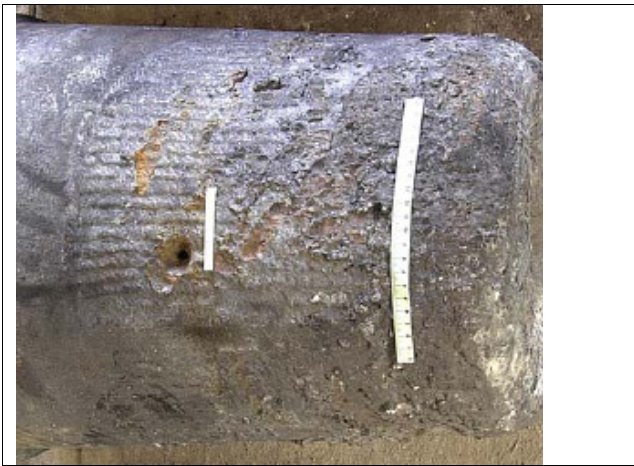
Figure 2: A tuyere showing defect in the form of small holes on its front part
