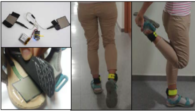
Fig 1. (left) Front and back FSR, accelerometer and battery; Sandal with back FSR (right) walk and thigh stretch movement.
