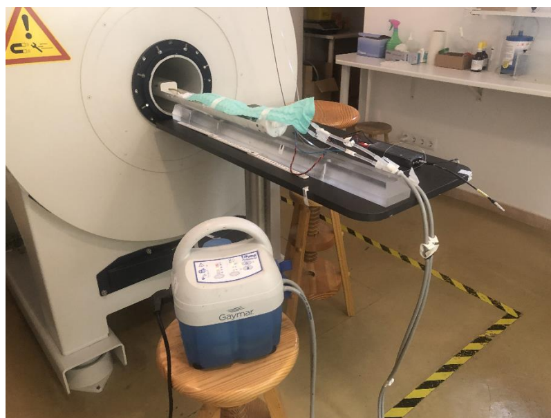
Figure 14. Circulating warm water pump (white and blue) and heat blanket (green) placed on the animal.
