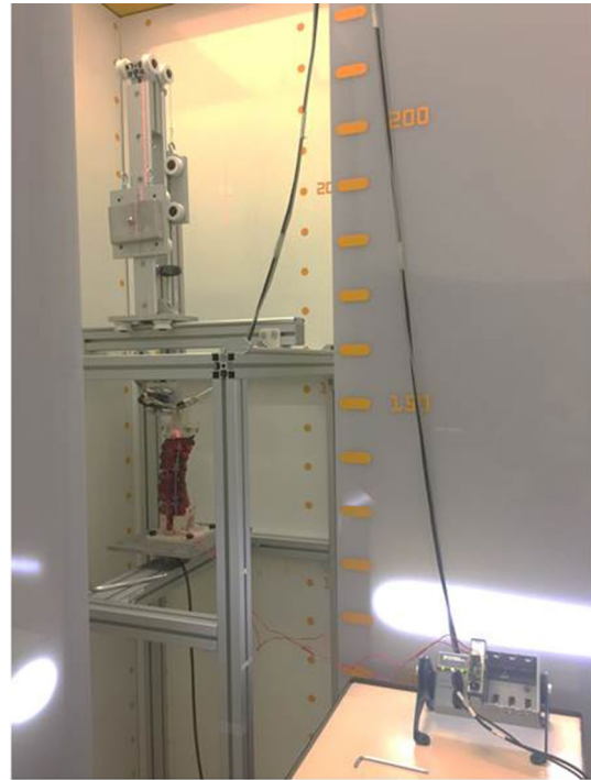
Fig. 2 Specimen mounted on the specially designed testing apparatus equipped with an EOS imaging system for motion tracking
