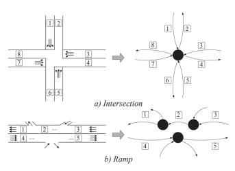
Figure 4 – An example of road network element represented by weighted complex network (number labels in the figure are identifiers of road section)
