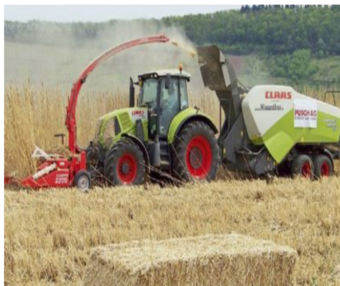
Figure 4. Production of chopped and baled biomass with forage harvester and modified baler
