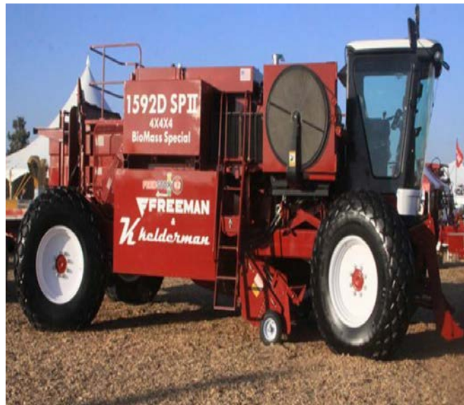
Figure 2. Self-propelled baler (Freeman: model 1592D Big Baler)
