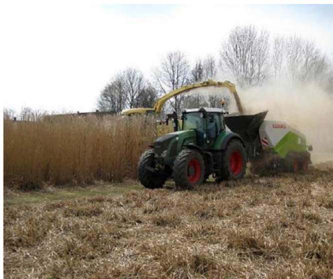
Figure 3. Production of chopped and baled biomass with SPFH and modified baler
