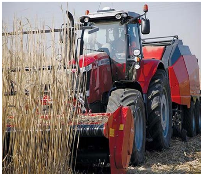
Figure 1. Harvesting and baling with front shredder and baler (Kuhn: WS 320 BIO shredder)
