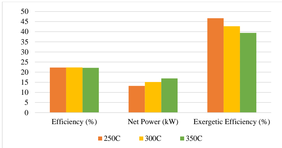
Figure 3: ORC Performance: thermal efficiency, net power and exergetic efficiency.
