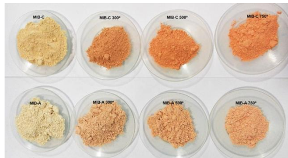
Figure 4.3.2 – Portuguese kaolins MIB-C A and MIB-A as natural and in different calcination temperatures.
