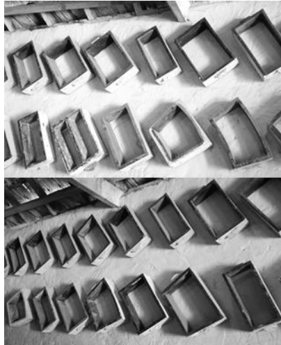
Figure 3.3.2 – Typical wood adobe molds.
