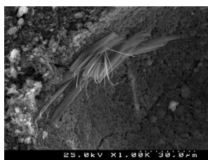
Figure 4.1.11 - SEM image with the efflorescences formation evidence (2.1 NaOH, 180 days of cure).
