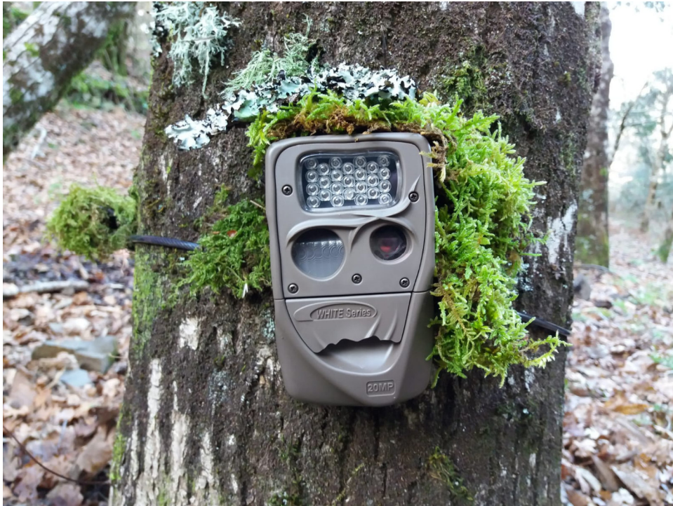
Figure A1 - Example of a camera trapping station (Cuddeback 20 Megapixel IR H-1453 white series).
