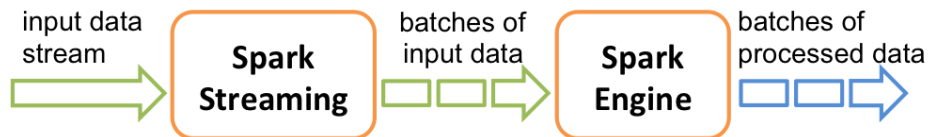
Image 21- Spark streaming and Spark engine relation
