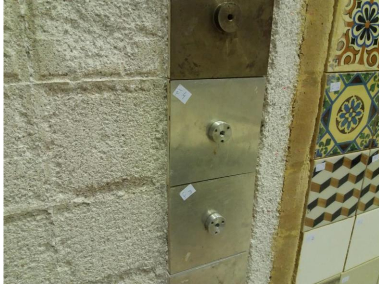
Figure 7 - Metal plates glued in tile glaze.
