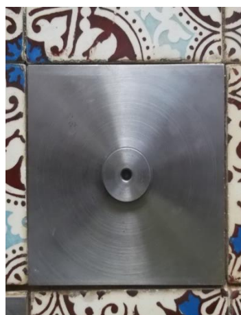
Figure 9 - Metallic plate glued into tile
