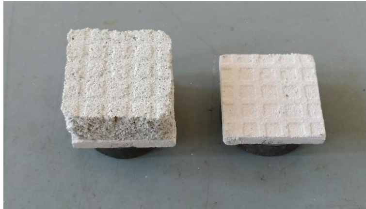
Figure 4 – Rupture applications test of mortars in tiles.
