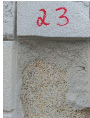
Figure 3 - cut in NHL body with 16 \pm 2 mm of depth (CC)
