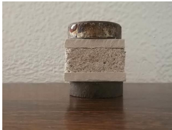
Figure 2 - Adhesion strength test specimen
