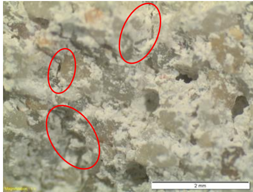
Figure 7 - Image at stereozoom microscope of mortar A with 90 curing days
