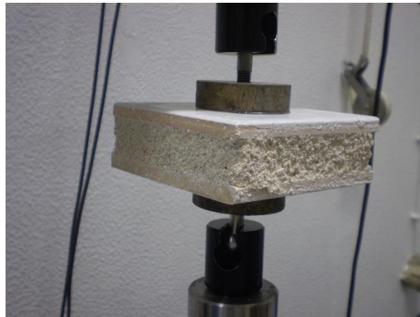
Figure 3 - Adhesive strength test specimen
