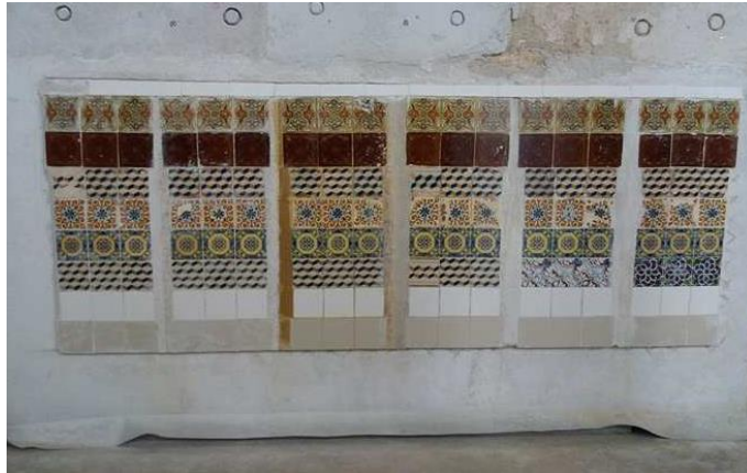
Figure 8 - Interior wall after accelerated curing cycles
