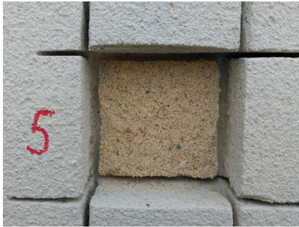
Figure 2 -cut in NHL/air mortar interface (CI)
