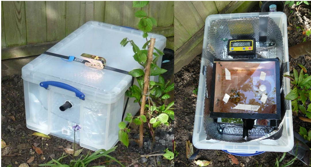
Figure S1. Insulated field box containing a young Bombus terrestris colony at time of placement in the field. Boxes contained a data logger connected to scales on which the colony box was placed; the colony was connected to the outside by a plastic pipe.
