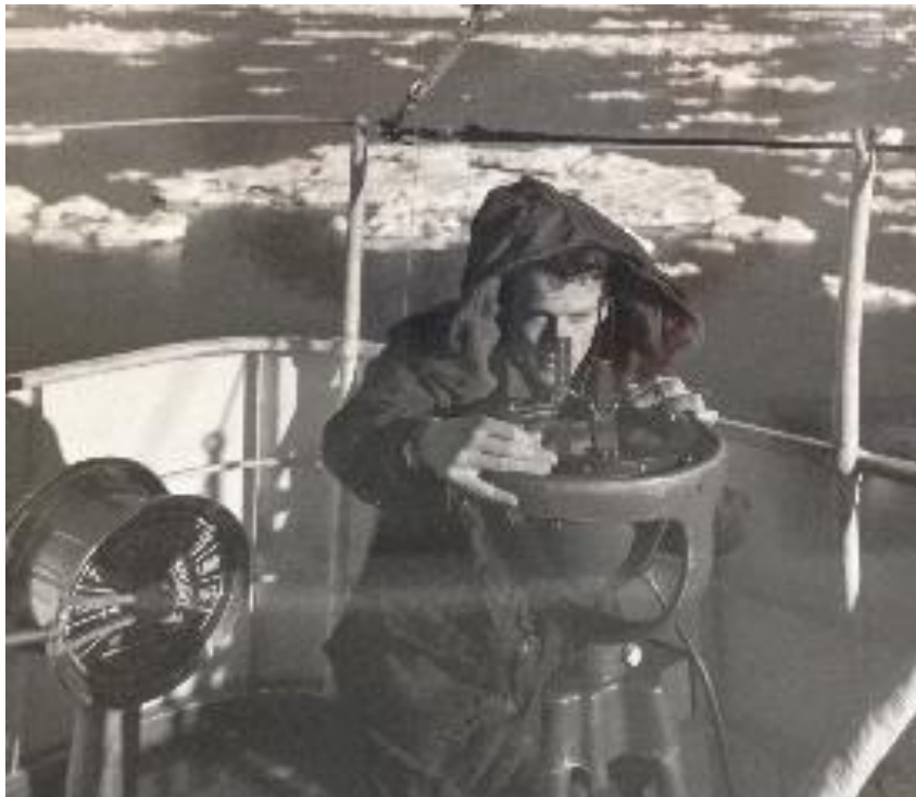
Figure 4.17: 'From the upper bridge of the C.D. Howe , Hydrographer, Steve Murphy, of the Department of Mines and Technical Surveys, "takes a fix" to determine the exact position of the ship in the Ungava Bay.' Wilfred Doucette, 1951, National Film Board of Canada collection, C.D. Howe . Source: Library and Archives Canada, accession 1971-271 Box 77, Item 59662.
