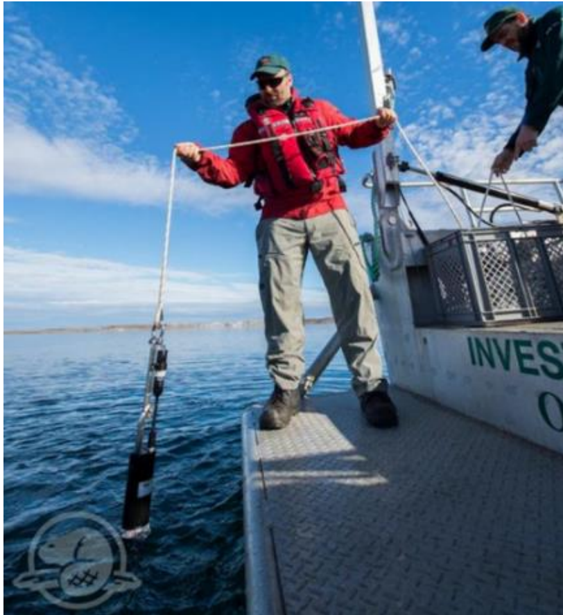
Figure 5.22: 'Filippo Ronca and Parks Canada UAT Diver, Ryan Harris lowering a sound velocity probe into water to scan for HMS Terror in 2016.' Copyright Parks Canada. Source: Parks Canada, 2016.
