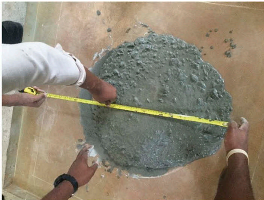
Figure 6. (a) Slump flow test; (b) a V-funnel test.
