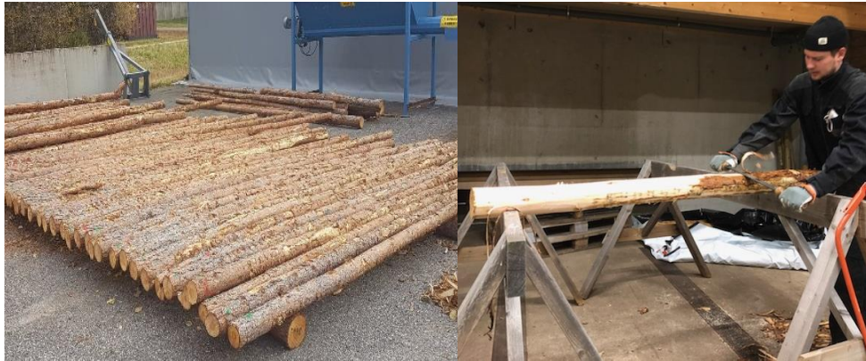
Figure 2. Left: Experimental logs during storage. Right: Manual debarking of logs. (Photo: Atanu kumar das)
