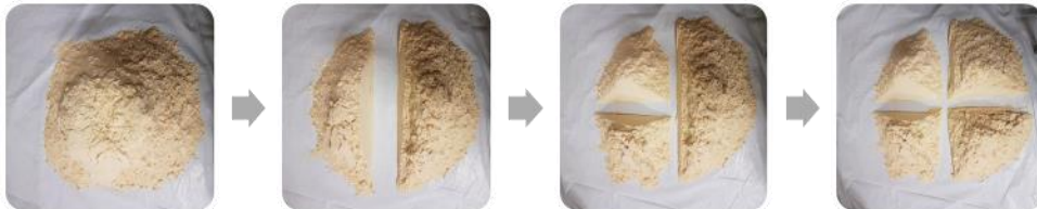
Figure 4. The wood powder sampling process, "The coning and quartering method". (Photo: Tobias Holdo)
