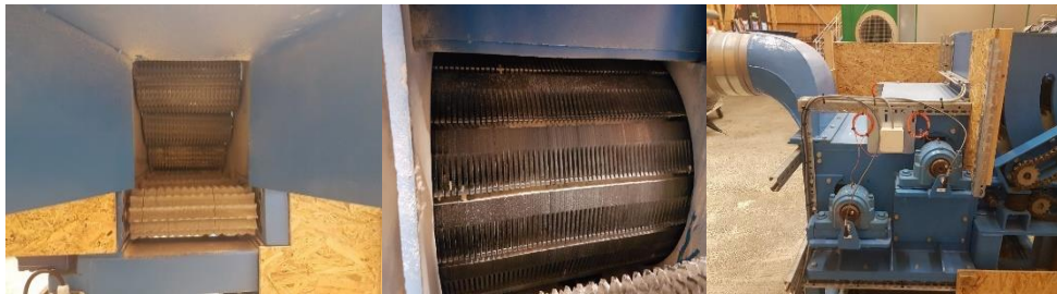
Figure 3. Left: Feeding conveyors. Centre: Multi-blade roller. Right: Profile view of the mill and its two multi-blade rollers. (Photo: Tobias Holdo)
