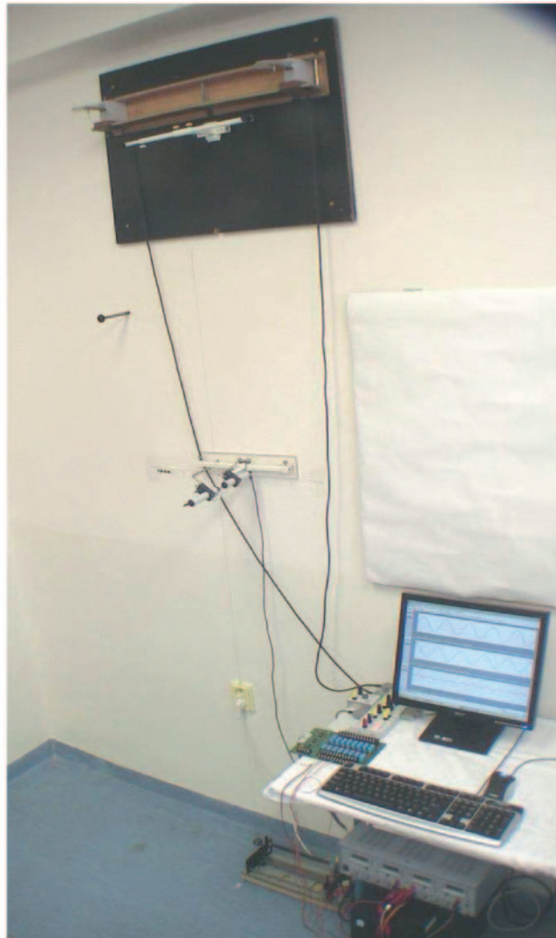
Fig. 4. – Arrangement of the experiment Mathematical pendulum.
