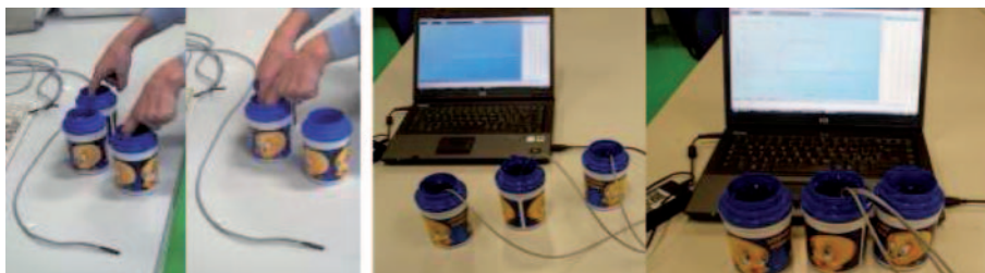
Fig. 4. – Locke's experiment using the fingers and temperature sensors.
