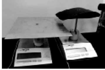
Fig. 6. – The double scale experiment: lower weight on the right (lift) higher weight on the left (downwash).
