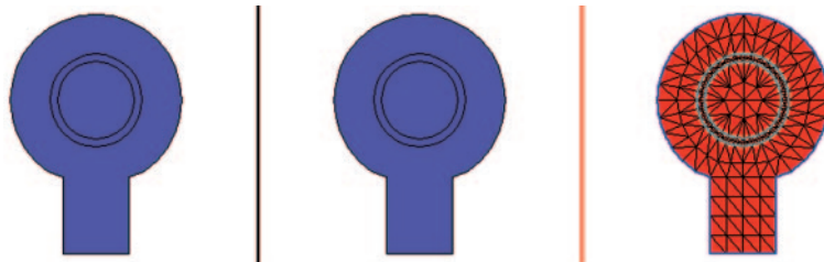
Fig. 3. – Computational domain. Left and middle: simulation domains for cytosolic calcium and ER-calcium, respectively. Right: coarse grid for finite-volume discretization of the underlying PDEs. In the multigrid method this grid functions as the coarsest grid on which a hierarchy of refined, interleaving grids is computed.
